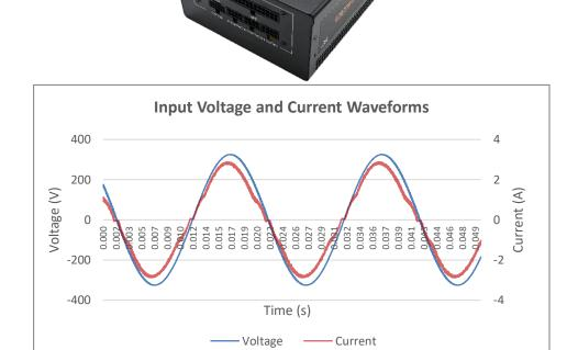
Input AC Current Waveform (ITHD = 7.07%, 50% Load)
