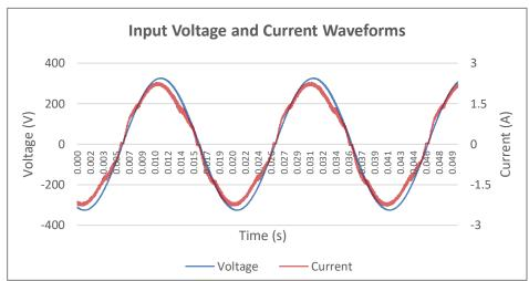
Input AC Current Waveform (ITHD = 5.89%, 50% Load)
